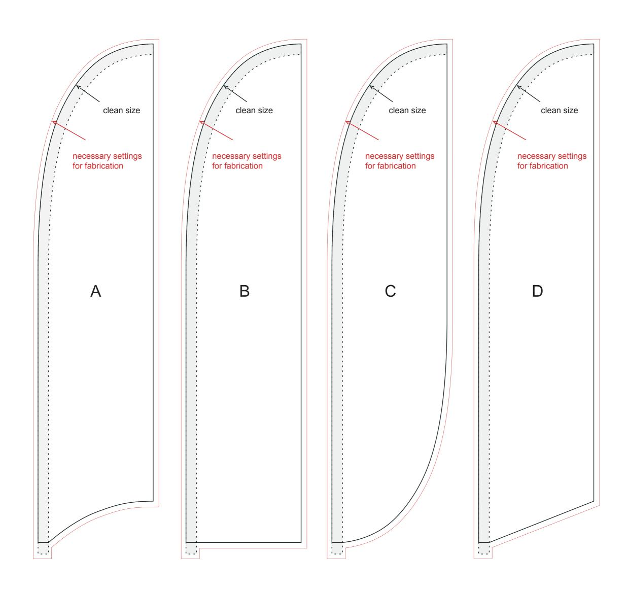
The grey arc in the template shows the underlay and stitching of the rod tunnel - we do not recommend placing smaller graphics, texts or logos in this space, as they could be slightly deformed by stitching.
