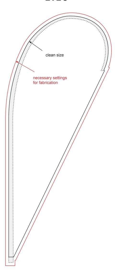
The grey arc in the template shows the underlay and stitching of the rod tunnel - we do not recommend placing smaller graphics, texts or logos in this space, as they could be slightly deformed by stitching.
